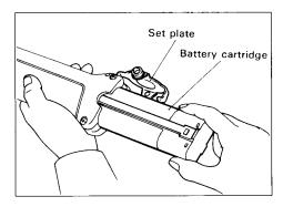
Do not use force when inserting the battery cartridge.
